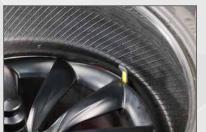
The mounting phase of the second bead is completed with the **simultaneous use of the bead breaker disc**, the rotation of the turntable and **in the presence of lowered tyres or RFT** with the use of the Press Mate which ensures that the tyre remains in the rim channel.
