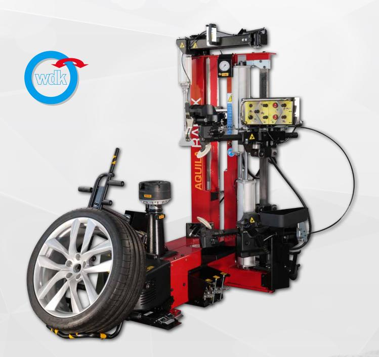
Super Automatic tyre changer with technology "SENZA LEVA" - CONTACTLESS Innovative super automatic tyre changer for all wheels from 13" to 28"
