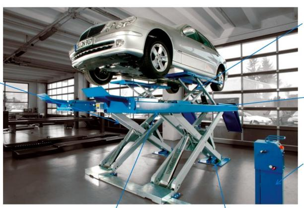
Whee-free lift with adjustable lifting platforms and NT Technology
