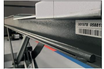
Includes sliding guide for Jacking Beams.
