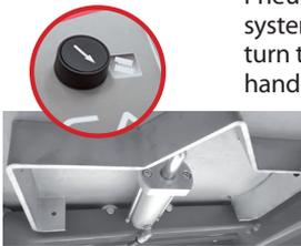
Pneumatic blocking system of alignment turn tables for easier handling.
